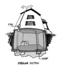
usually reduced by one of four types of soil suction: subslab suction, drain tile suction, sump hole suction, or block wall suction. Active subslab suction (also called subslab depressurization) is the most common and usually the most reliable radon reduction method. One or more suction pipes are inserted through the floor slab into the crushed rock or soil underneath. They also may be inserted below the concrete slab from outside the house. The number and location of
