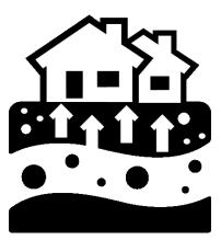
adon is a naturally occurring radioactive gas produced by the breakdown of uranium in soil, rock, and water. Air pressure inside your home is usually lower than pressure in the soil around your home's foundation. Because of this difference in pressure, your house acts like a vacuum, drawing radon in through foundation cracks and other openings.
