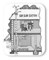
prevent radon gas from entering the home from below the concrete floor and from outside the foundation. DEP-certified radon mitigation contractors may use other methods that may also work in your home. The right system depends on the design of your home and other factors.
