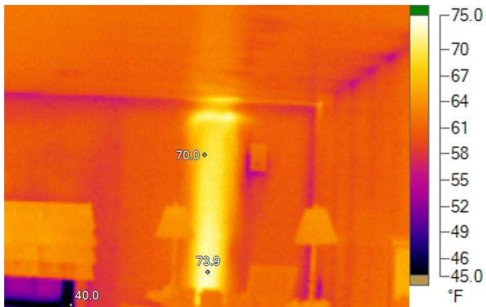
IR001061.IS2 12/18/2009 10:16:45 AM Image displays heating duct in wall to bedroom
